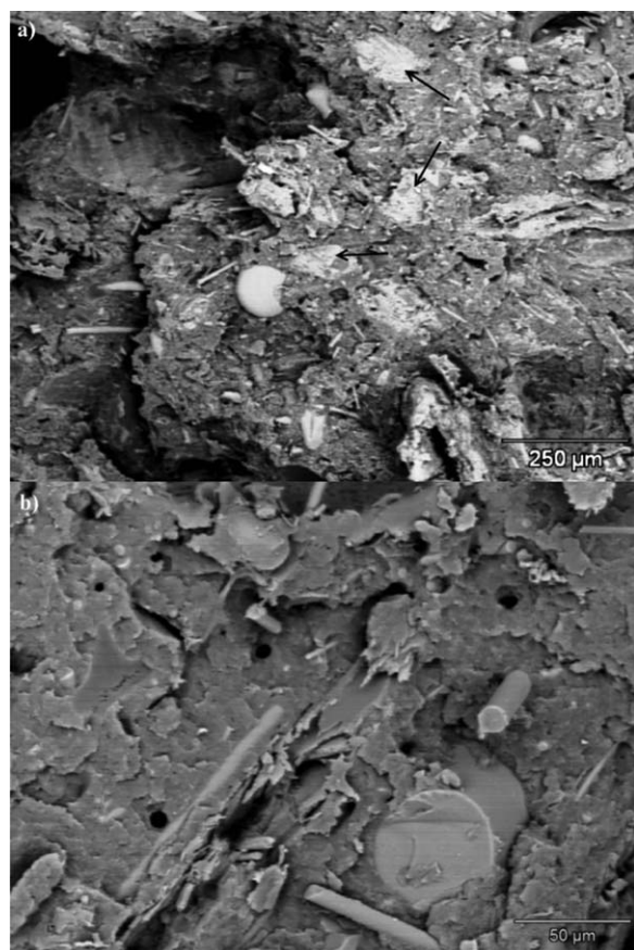
Figure 7. SEM micrographs of the WF-PP-MW-PB composites at magnifications of (a) 100 and (b) 500 \times .
