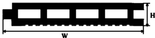
Figure 5. Hollow profile of an extruded WPC with a width ( W ) of 126.0 mm and a height ( H ) of 20.0 mm.
